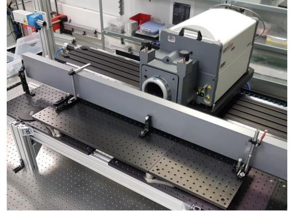
ALBA stitching interferometry platform, for sub nm metrology of large optical elements
