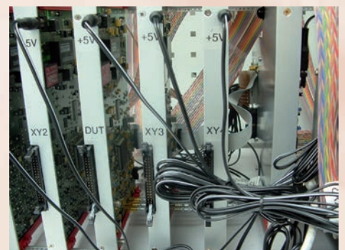
Partial view of a particle telescope with 4 planes based on the Alibava System
