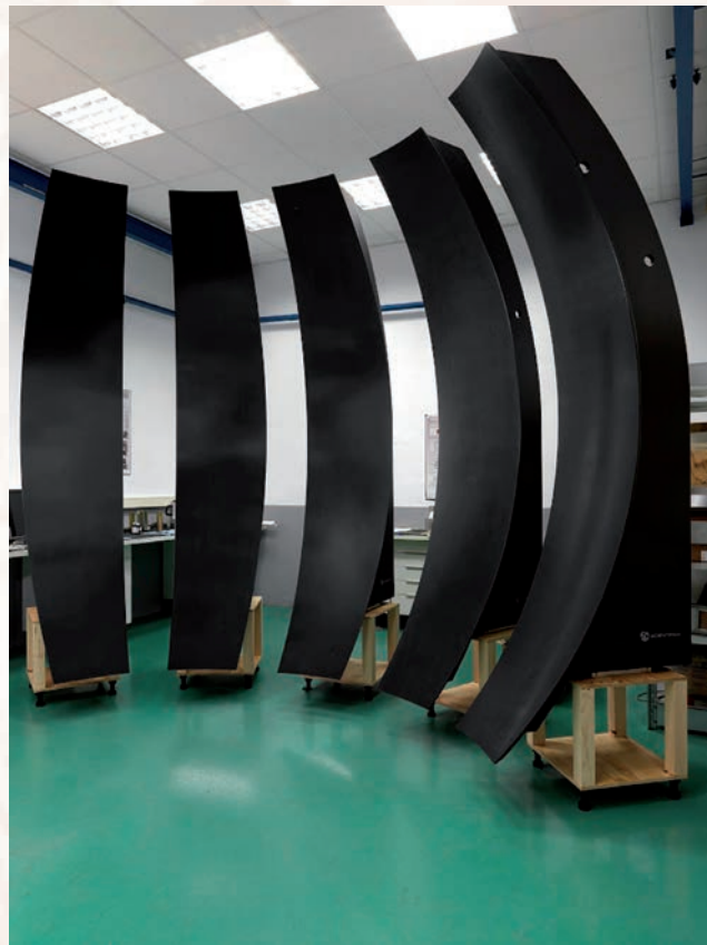
Units of neutron back-scattering analyzer's support structures made in carbon fiber, for IN16B instrument at ILL
