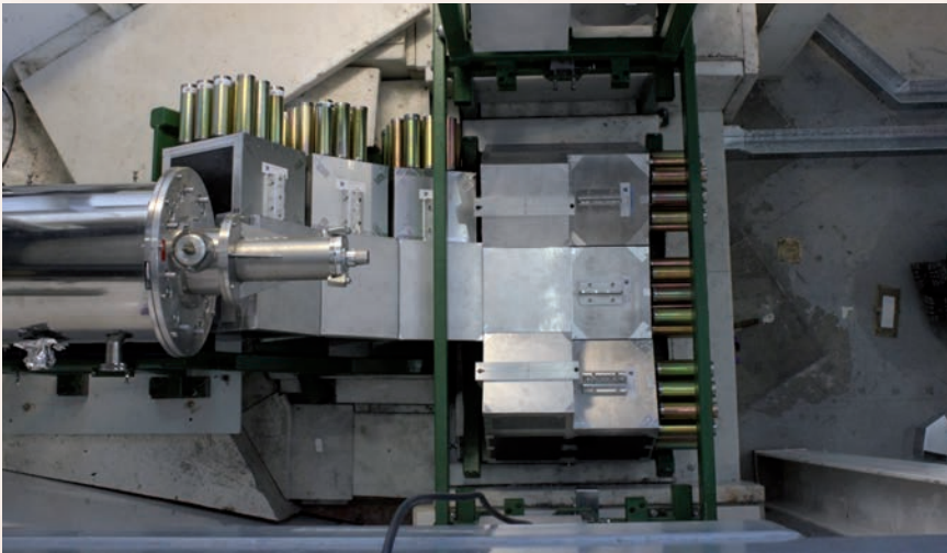
High Pressure neutron diffractometer (PEARL) at ISIS, UK. Position sensitive neutron detector modules during instrument installation
