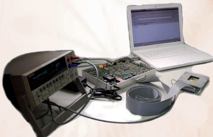
Particle detector readout Alibava System with 256 channels
