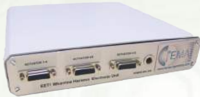
[ESO] Controller for the Warping Harness Prototypes for positioning hexagonal mirrors of the EELT telescope, 2009
