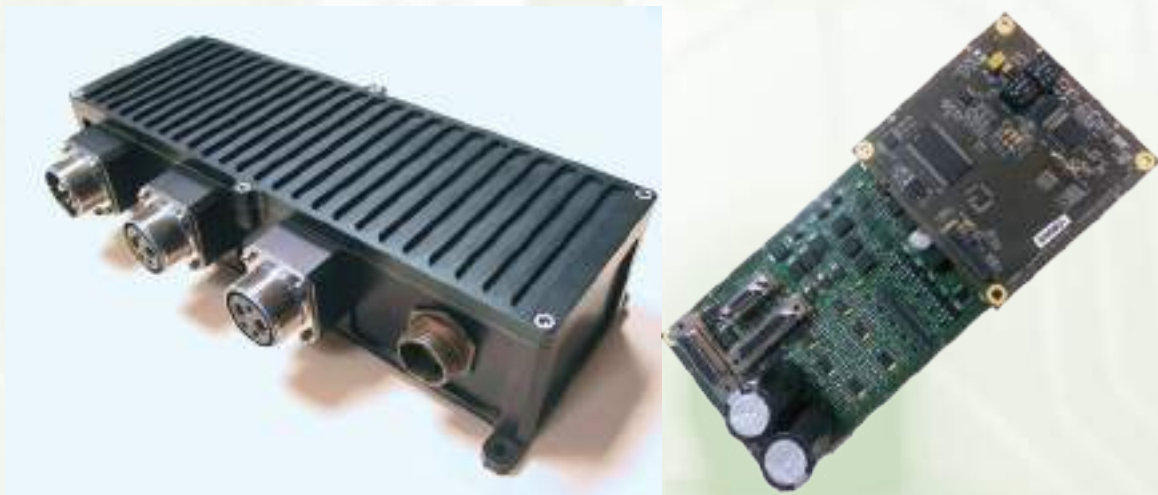
[Airbus DS] Equipment for 270Vdc High Voltage Distribution in aircrafts, 2012
