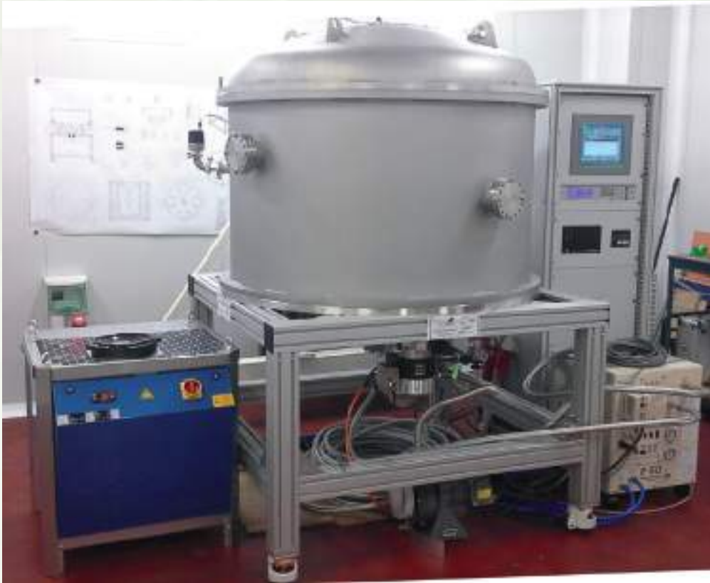
[INTA] Design, manufacturing and supply of a cryostat for 4° Kelvin, for optical and mechanical testing of components of the ESA/SAFARI instrument, 2013
