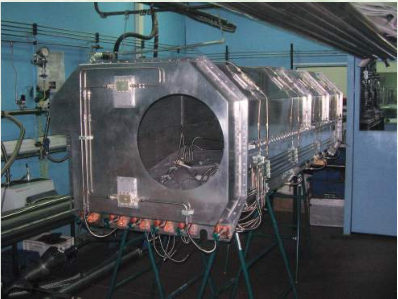
[IAA] CARMENES in-vacuum cooling hardware, 2014
