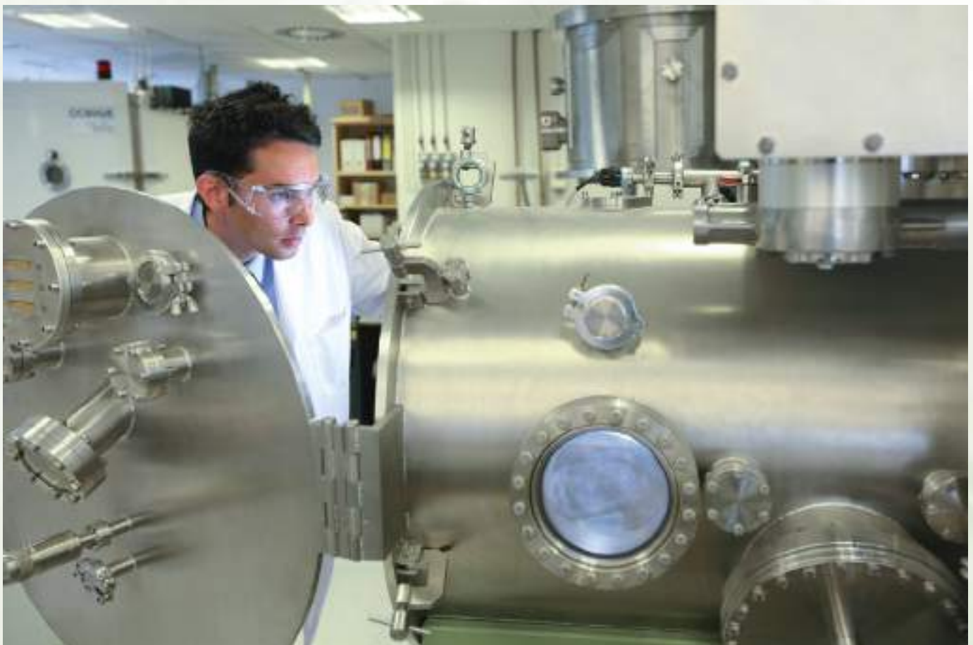
TRIBOLAB station for the study of solid lubricant coatings for aerospace applications
