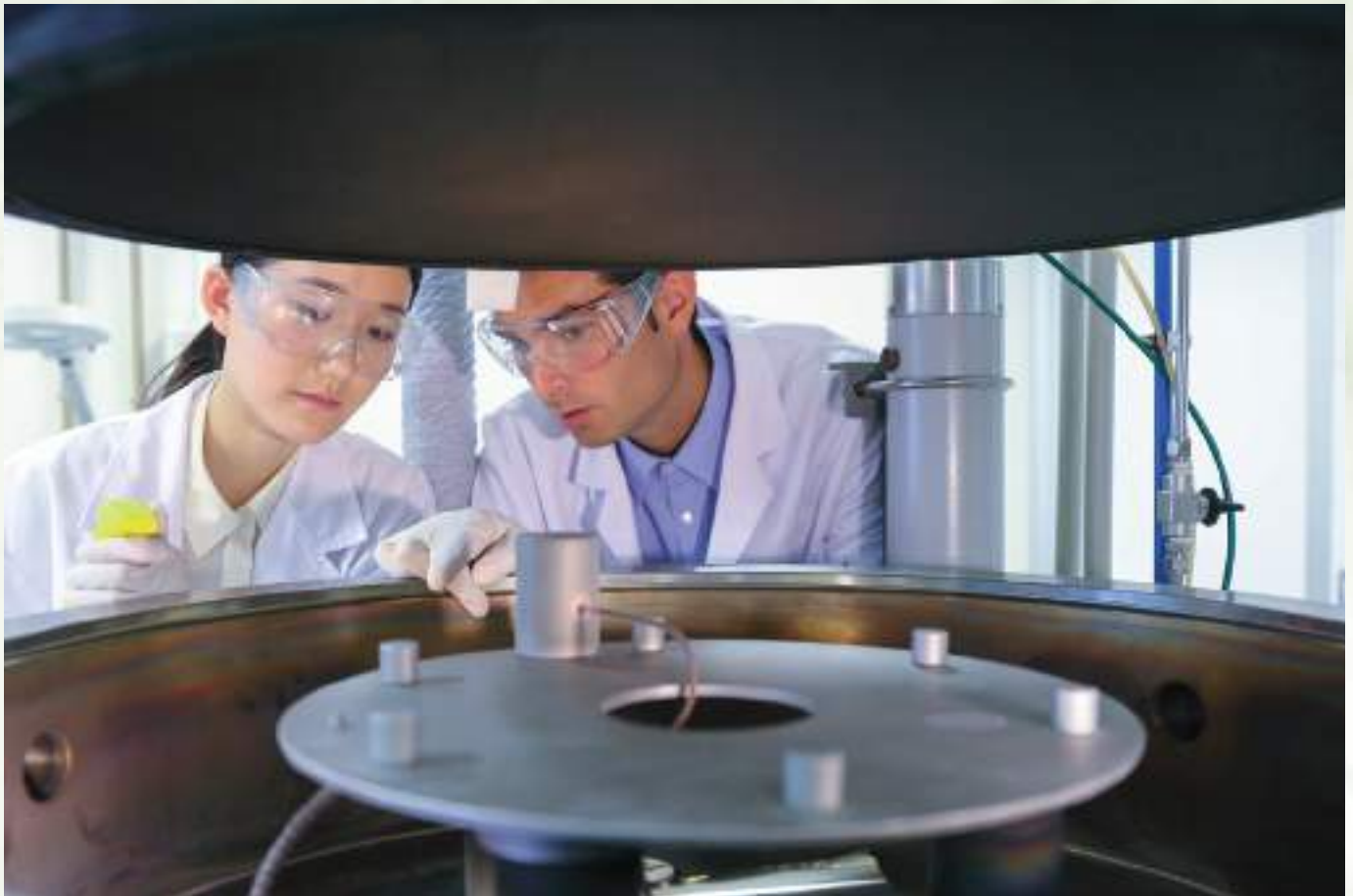
Laboratory for Advanced Surfaces. Semi-industrial plasma nitriding by active screen or post-discharge (ASP) equipment.
