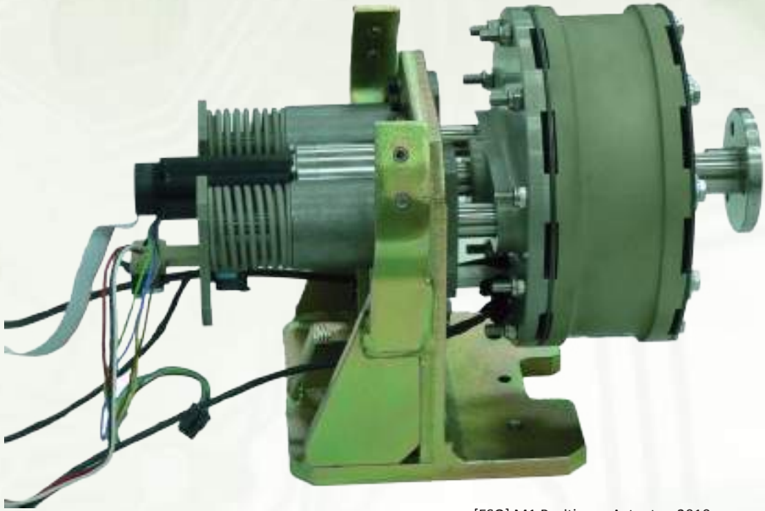
[ESO] M1 Positioner Actuator, 2010
