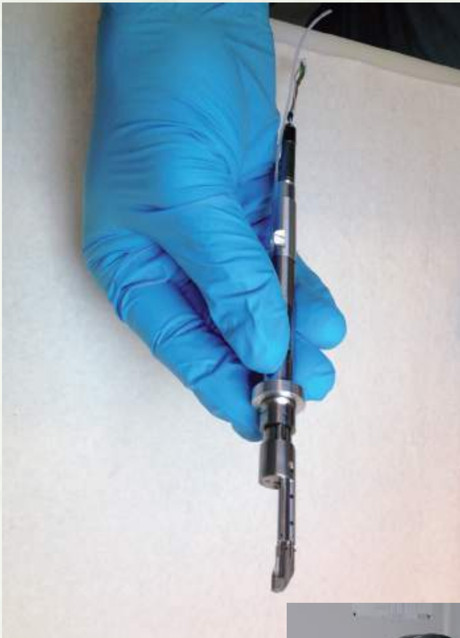
[INTERNAL FUNDING], Design, manufacturing and integration of a 10mm pitch fiber positioner robot, 2012
