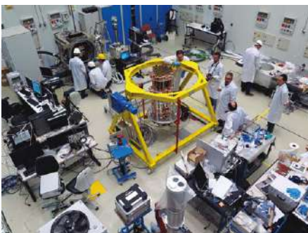
Integration in the AIV room of the TGI (Thirty Gigahertz Instrument), the second instrument for the QUIJOTE Experiment, at theTeide. © Pablo López /IAC.
