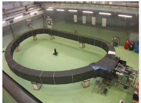
Toroidal Field Coils for ITER F4E
