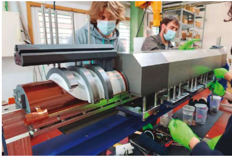
Fabrication of the MCBXFA for the HL-LHC
