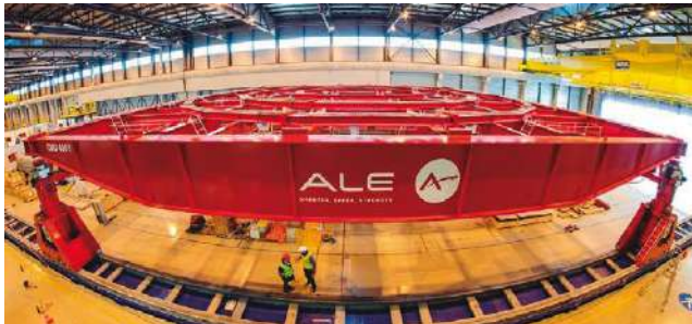
Gantry crane PF coil
