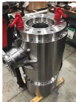
ESS Shaft rotatory unit
