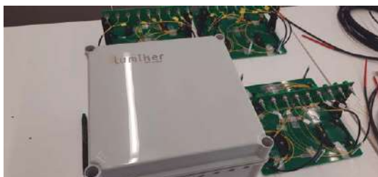
Optical Fiber Multiplexer
