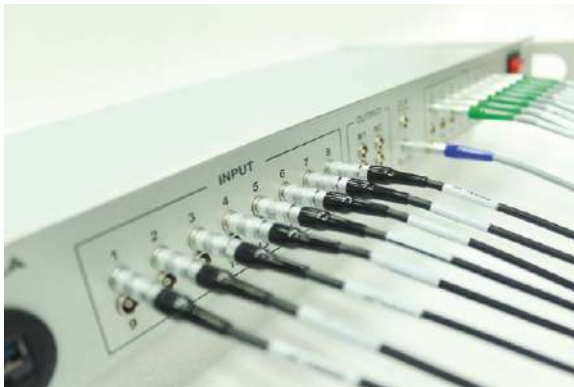
16 channels Digital Signal Processing System (FPGA)
