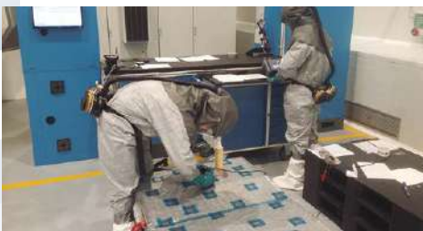
UT inspection of First Wall Pannels prototypes (ITER)
