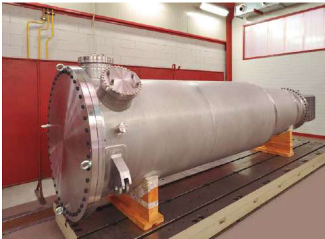
Proton Beam Window Port Block and Proton Beam Window Vessel for European Spallation Source ERIC
