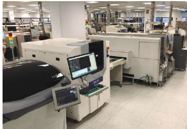
3 SMD component assembly lines
