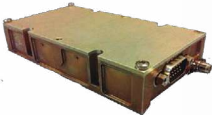
Photonic RF analogue link for space applications
