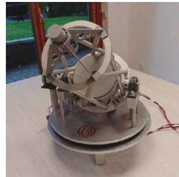
Scaled prototype for testing of control and actuation strategies for the EST main structure
