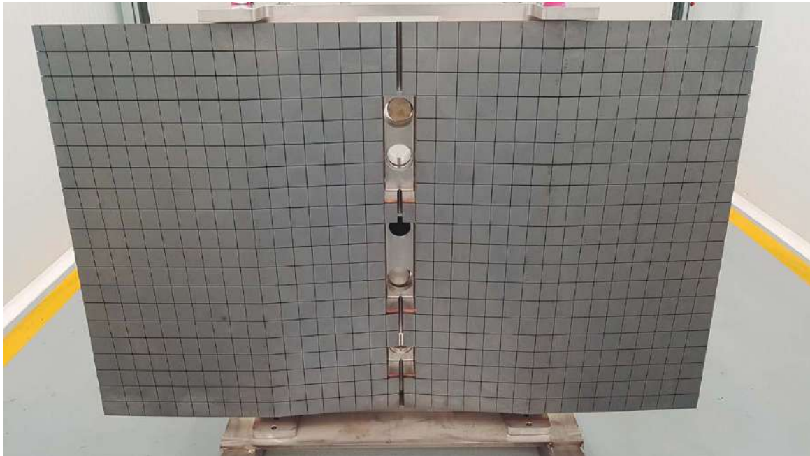
Finished First Wall Panel Semi Prototype
