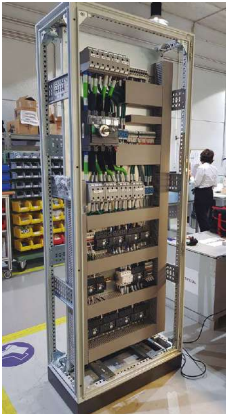
HSB01 distribution board
