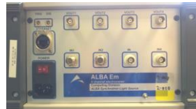
ALBA Electrometer: pA-mA high current precision reading
