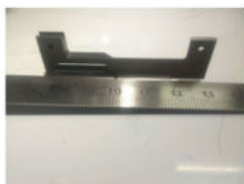
Special insert (CTE-matching with Si)
