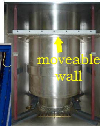
Output cavity (below tetrode)
