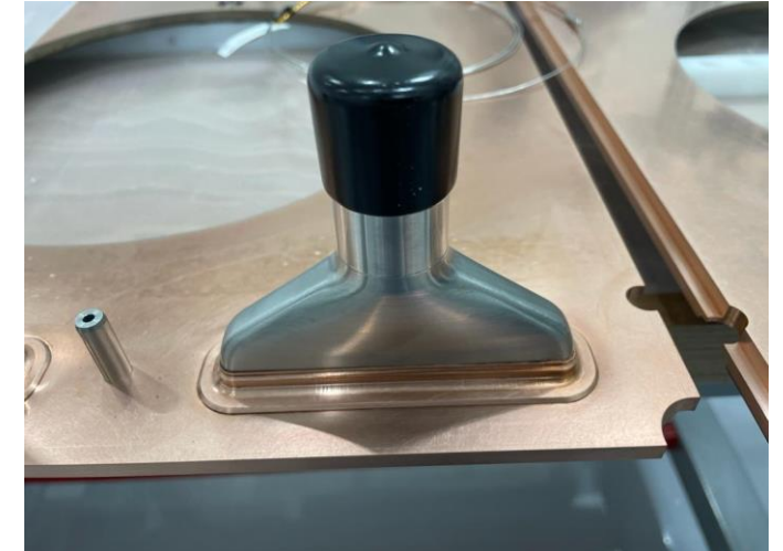
Heterogeneous joint between SS conveyor and exploded bonded Cu-Mo substrate
