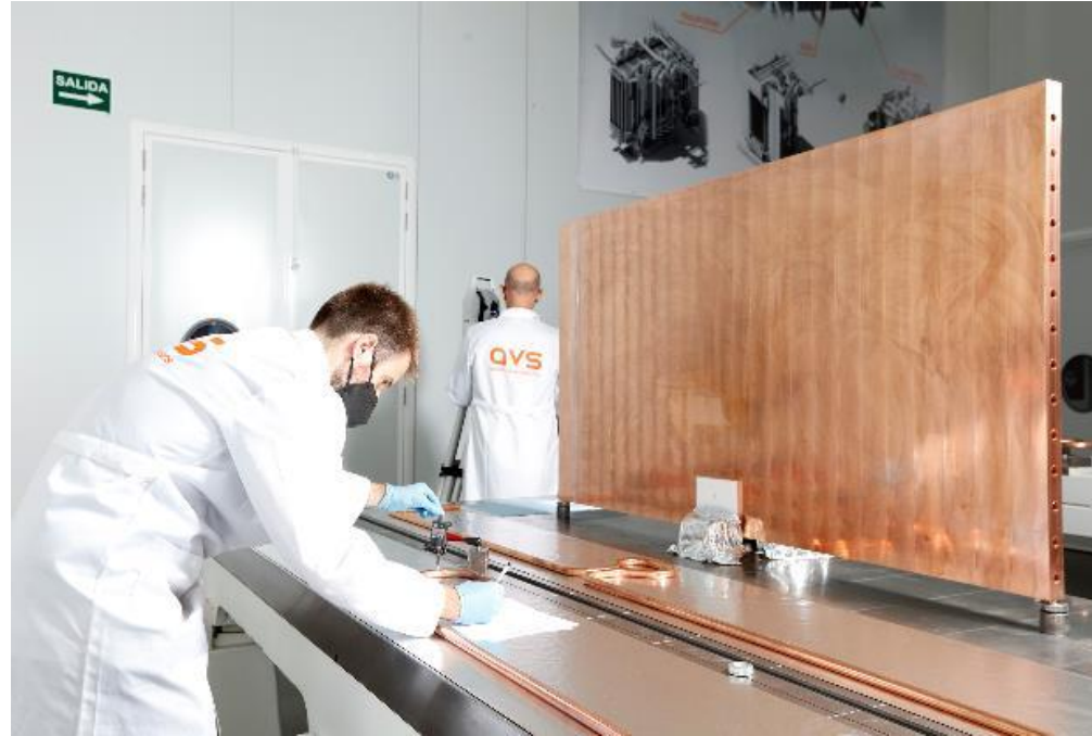
Deep drilling of Neutralizer panels completed Dimensional measurement of Calorimeter swirl tubes on-going
