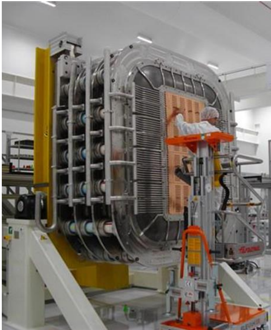
Alignment over the 1280 apertures of the accelerator stages with few tenths of mm precisions
