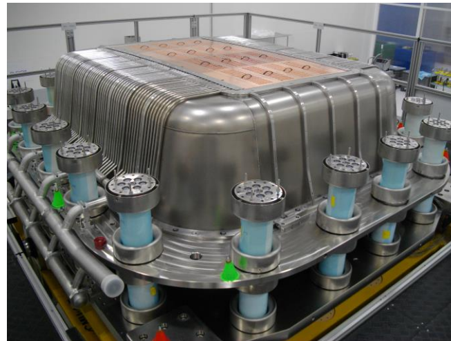
Assembly of one accelerator stage and its post insulators
