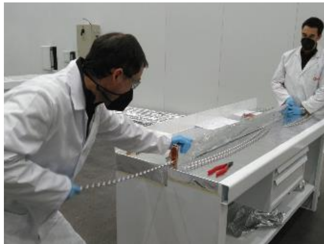
Insertion of twisted tapes completed for Residual Ion Dump
