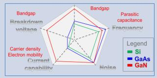
GaN allows to manage high power systems in a very efficient way, decreasing the total system loses, while operating in harsh radiation & magnetics environment.
