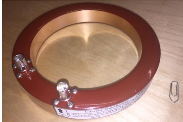
AC Current transformers
