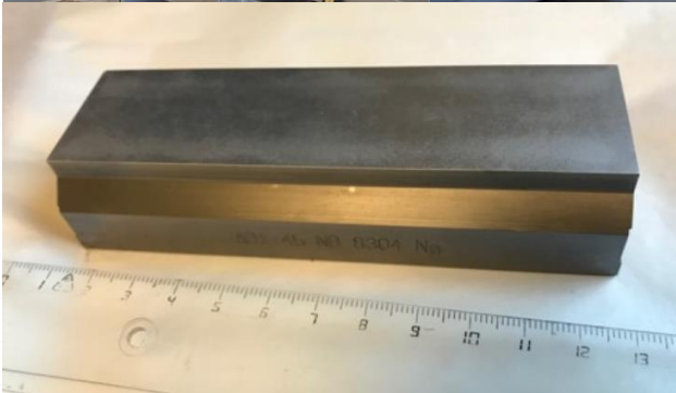
↑ Mo - graphite absorber block
