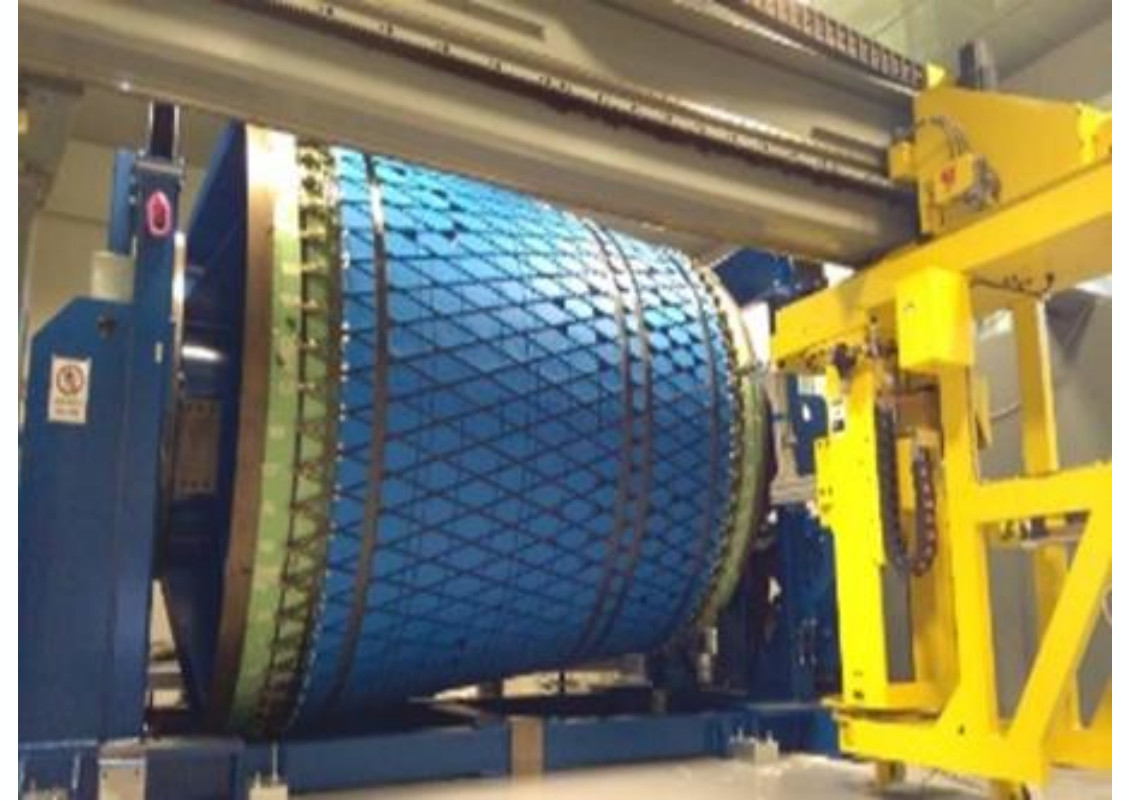
The interstage 2-3 of VEGA C Launcher manufactured using a composite grid structure technology
