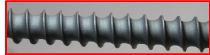
Screw coated with hydroxyapatite (HA)
