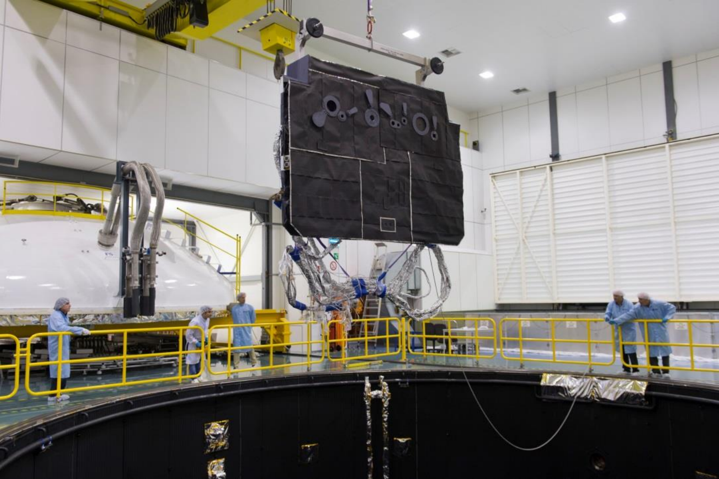
(left) Full size Heat shield entering the large space simulator at ESA (Right) under test
