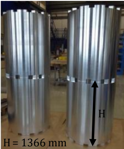
← Forged Al 7075 T6 for the shells of the MQXF quadrupoles
