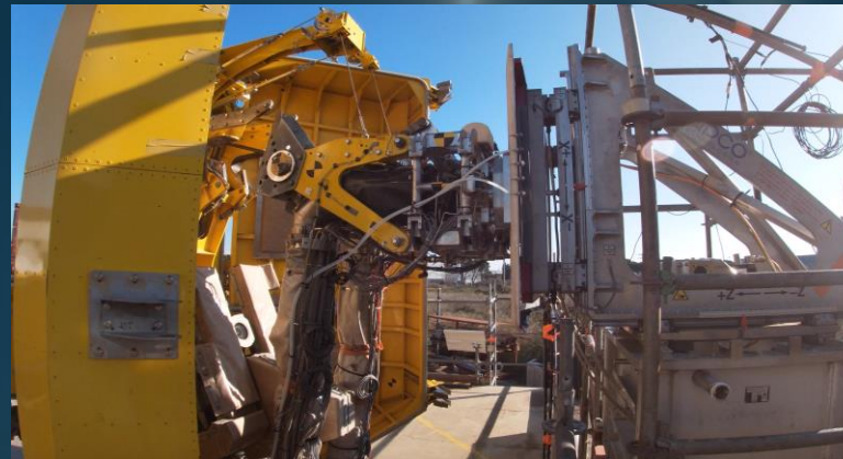
ECT on Cryogenic Connection Systems (CCS) disconnection and retraction tests
