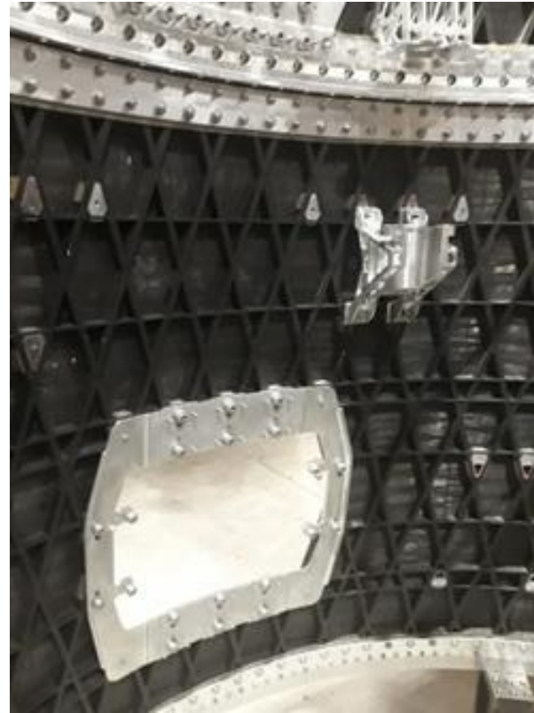
The interstage 2-3 of VEGA C Launcher manufactured using a composite grid structure technology
