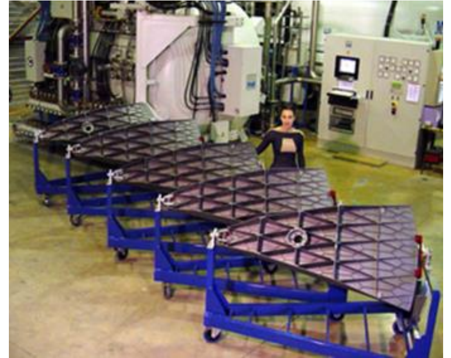
Herschel Space Telescope primary mirror integrated (left) and the constituent SiC petals (right), the largest ever build with the selected manufacturing process.
