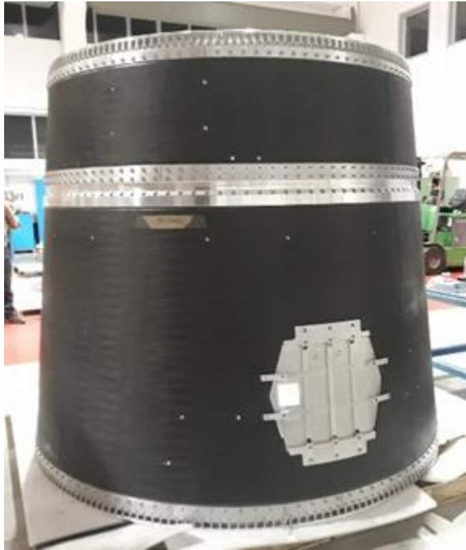
The interstage 2-3 of VEGA C Launcher manufactured using a composite grid structure technology
