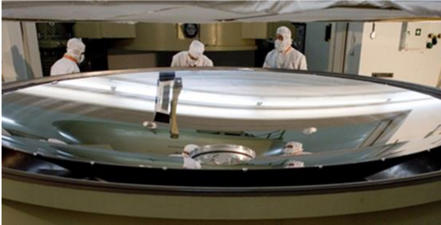
Herschel Space Telescope primary mirror integrated (left) and the constituent SiC petals (right), the largest ever build with the selected manufacturing process.
