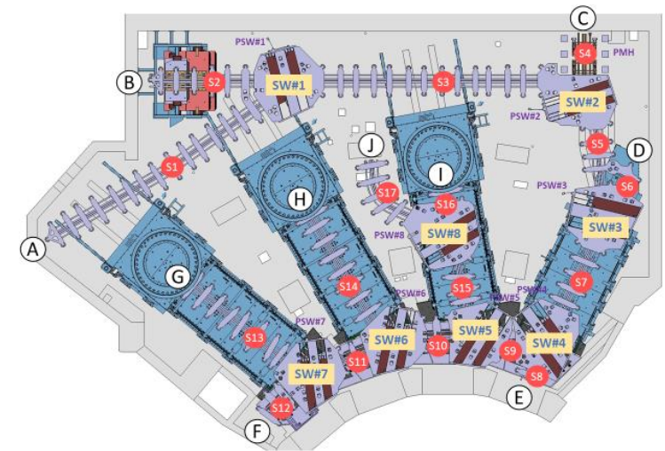
Monorail layout overlapped with the NB Injectors
