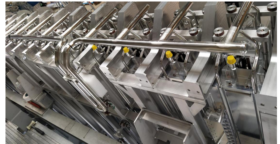
Prototype Neutral Beam cryopump assembly for the Mitica facility
