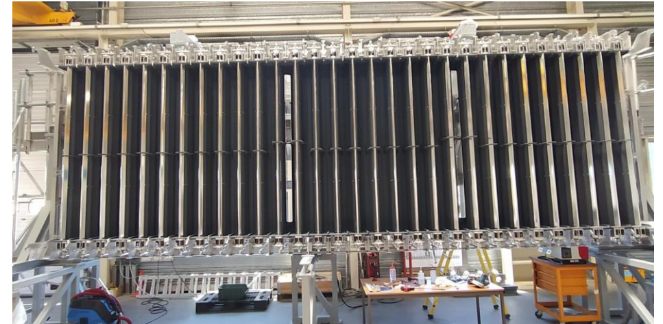
Prototype Neutral Beam cryopump assembly for the Mitica facility
