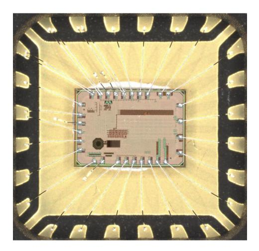
The TDC1001 is a radiation hardened time to digital converter with a single shot precision smaller than 8ps and zero dead time.
