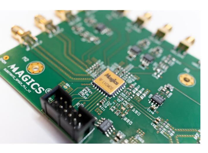
The PLL1001 is a radiation tolerant wideband phase locked loop (PLL), capable of delivering frequencies in the 1 MHz to 3 GHz range.
