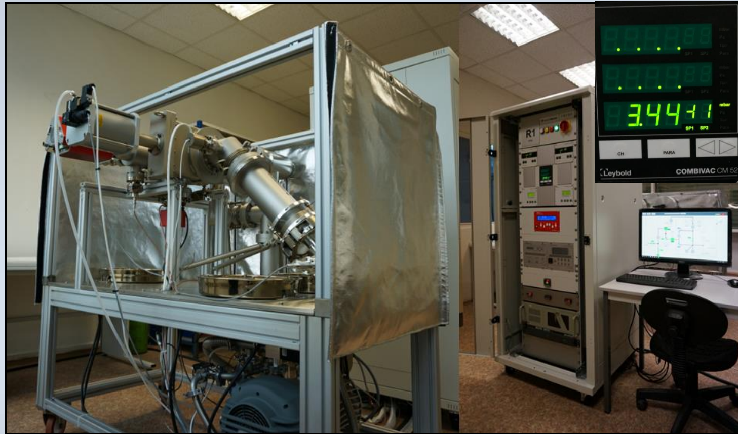
Pumping System for NICA Booster
