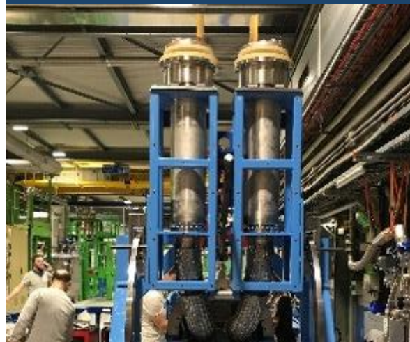
HL-LHC REBCO HTS Current Leads (up to 18 kA)
