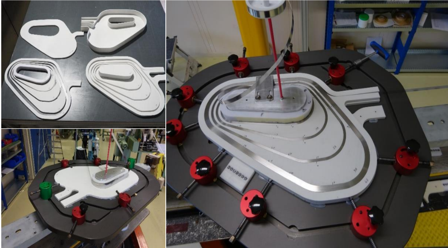
Stainless Steel dummy winding with 3D printed spacers
