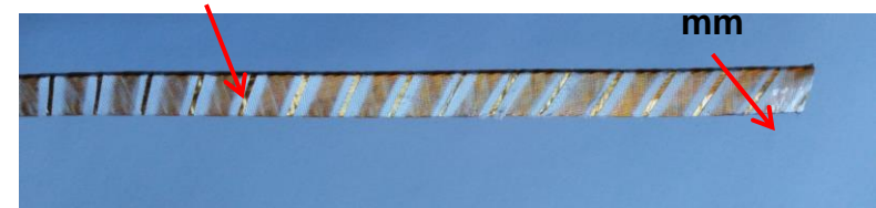
Fiberglass with an adhesive layer of 0,1 mm
