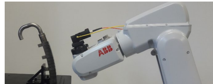
Reflectivity tests on PFC prototypes in support of IVVS optical design
