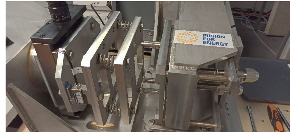
IVVS – Full-scale prototype of the Remote-handling Compatible Connector – it is the high-density electrical/optical connector assembly that services the IVVS Cartridge when installed; it must be connected/disconnected via remote tooling located in the CPRHS
