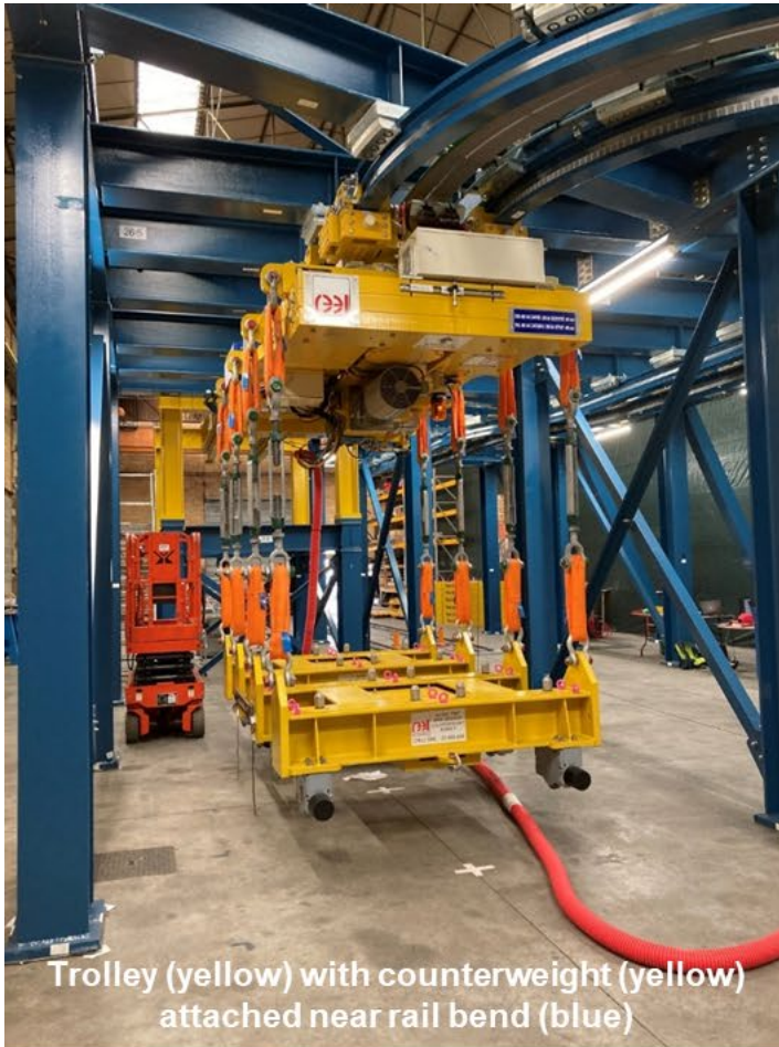
Small clearances due to space constraints in the NB cell
