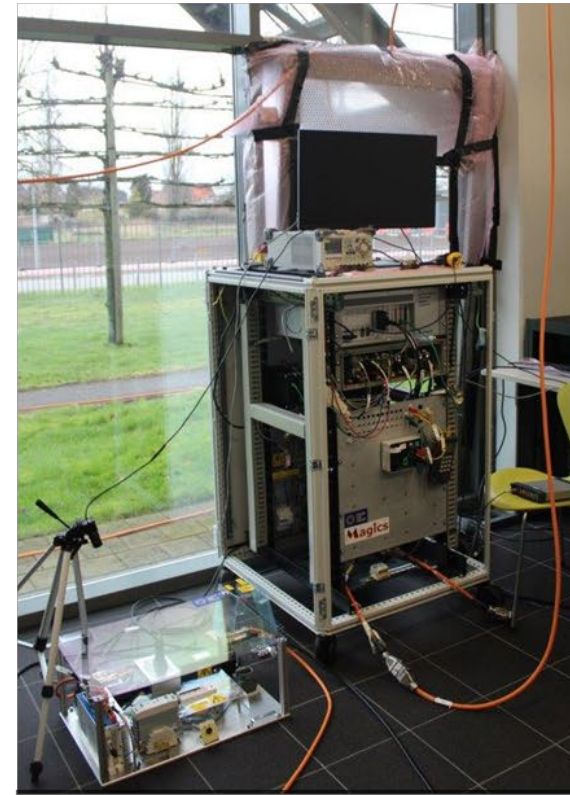
150-m cable communication tests for BISS module and irradiated ASICs (5 typologies)
