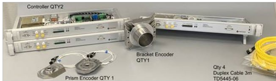
Special encoder for IVVS scanning head developed
