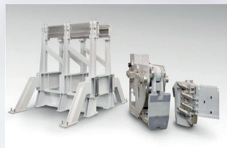
Divertor RH prototyping: CMM & SCEE lifting a dummy load
